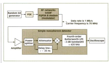
This noncoherent detector block circuitry was implemented for detector-output measurements.
