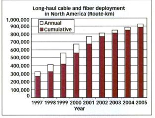
After reaching a peak of some 140,000 route-km in 1999, annual deployment of cable is expected to fall back to just under 35,000 route-km by 2003. With increasingly higher fiber counts cushioning the decline in terms of fiber-km, annual deployment of fiber drops from a peak of just over 10.8 million fiber-km in 2000 to approximately 7 million fiber-km in 2003.
