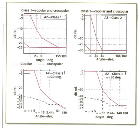
2. These are typical azimuth radiation-pattern masks proposed for LMDS antennas, using three classes of sectored base-station antennas (after ref. 4).
