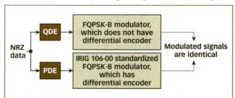
1. A special coding scheme, QDE without a differential encoder, is equivalent to the IRIG standard requiring a differential encoder.
