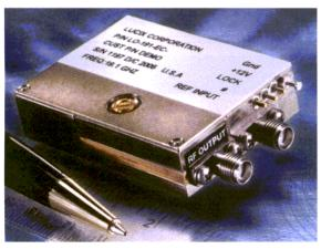
The desire for low noise Dielectric Resonator Oscillators to enhance clear communication, spectral purity, continues. Typical phase noise @ 100 KHz offset of -126 dBc/Hz for 10 GHz, -115 for 18 GHz, and -108 for 38 GHz are being measured on our production DROs. Harmonics measure between -50 dBc and -80 dBc. Spurious are less
