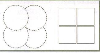
Traditional overlapping circular cells can be replaced with square cells for best results in an LMDS system. A specific antenna aperture distribution must be designed to accommodate this, however.
