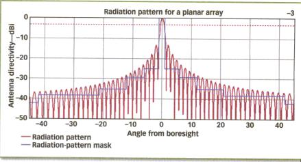
8. This is a normalized radiation pattern of an 80  $\times$  80 planar array of uniformly distributed isotropic sources compared to a sample radiation mask.
