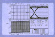
Bluetooth measurement tools range from powerful design analysis to fast, automated tests for the production line. Above, a modulation characteristics test verifies proper performance of the modulation circuitry to ensure reliable data transfer over the Bluetooth communication link.
