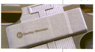
MEMS technology allows this miniature SPST microwave switch to operate over an extremely long lifetime with minimal RF performance degradation and power consumption.
