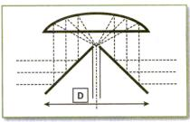
4. This conceptual design represents an omnidirectional antenna for LMDS base stations (after ref. 3).
