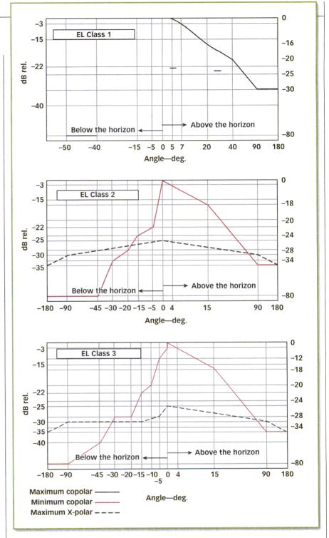
3. These are typical elevation radiation-pattern masks that were proposed for LMDS antennas, using three classes of sectored base-station antennas (after ref. 4).
