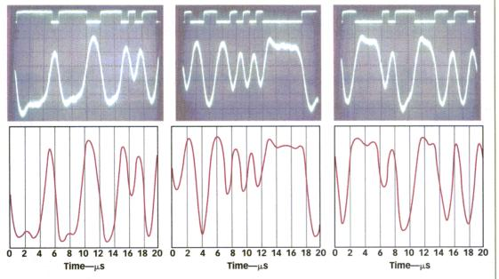
6. A comparison of actual (upper) and computer generated (lower) waveshapes of the noncoherent-detector output shows a close resemblance to one another.
