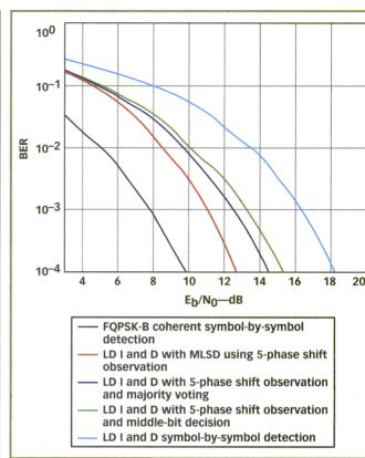
4. BER performance for various LD I&D noncoherent detection techniques is shown here.
